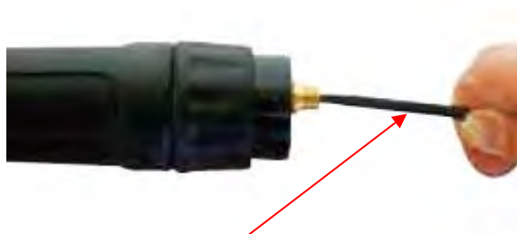
(3) Carefully pull out and completely remove the liner.
