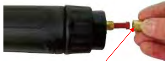
(2) Remove the liner retaining nut.
