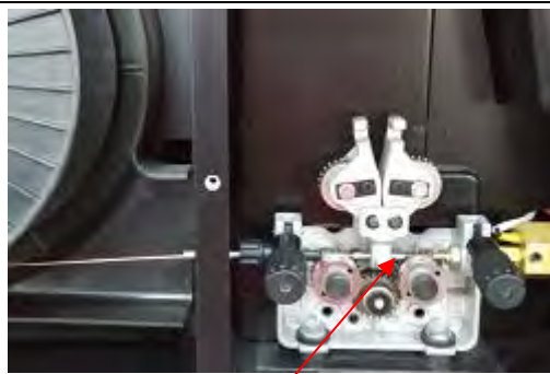
(12) Feed wire over the drive roller into the outlet guide tube, Push the wire through approx 150mm.
