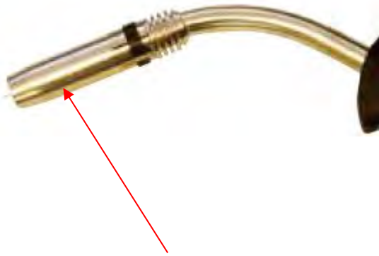
(17) Fit the gas nozzle to the torch head.
