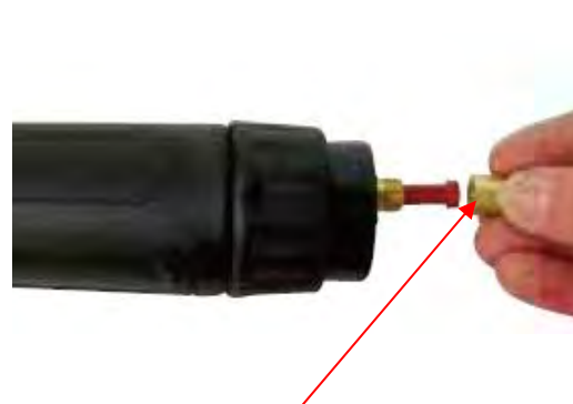
(2) Remove the liner retaining nut.
