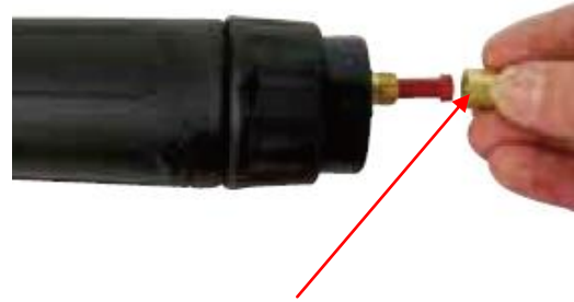
(2) Remove the liner retaining nut.
