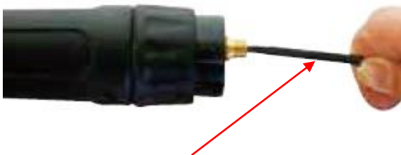
(5) Carefully feed in the new liner in short forward movements down the torch lead all the way to exit the torch neck. Be care-full not to kink the liner.
