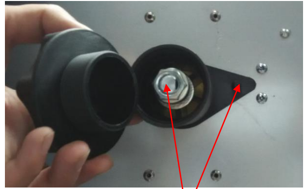
(2) Note the tension spring adjuster and spool locating pin.
