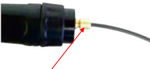
(6) Push the liner firmly into the torch lead
