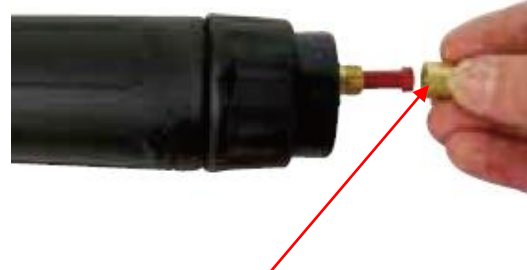
(2) Remove the liner retaining nut.
