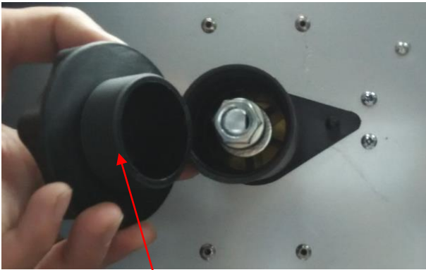
(1) Remove the spool retaining nut.
