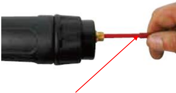
(3) Carefully pull out and completely remove the liner.
