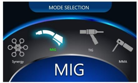
This page allows you to select welding methods as below: Synergy, MIG, LIFT-TIG, MMA
