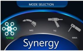
In the SYNERGY mode, the user only selects the basic welding parameters such as the type of material, the thickness of the material to be welded, and the diameter of the welding wire (0.8mm, 1.0mm and 1.2mm available). Other parameters of the device are selected automatically using the database of uploaded programs.
