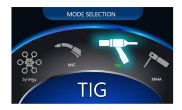
In the TIG (Tungsten Inert Gas) method, the electric arc strikes under an inert gas (argon) shield, between the welded element and the non-fusible electrode made of pure tungsten or tungsten with additives.
