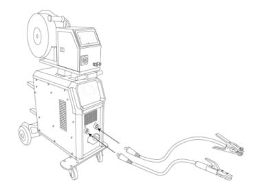
Connect the welding and mass leads to the appropriate output connectors of the welder, according to the polarity recommended by the manufacturer of the electrodes you intend to weld.
